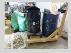
The pod trash collects on the screen and is removed from the cleaner with a shop vac. There is a little bit of work, some noise and dust, but it is high-throughput and can be operated by one person. I have used the R9 for several years now and have cleaned a lot of milkweed seed, besides a lot of other wildflower seed with lesser machines. This is fun to do, and I thank everyone who has helped collect seed, and those who helped plant seed. If you need seed for any reason, just let me know.
